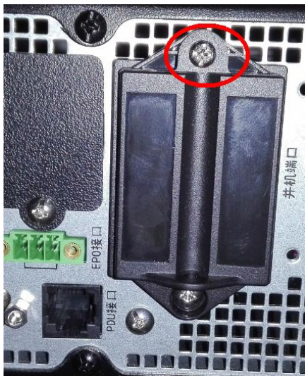
Step1. Unscrew the parallel cover.
