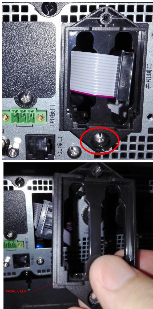
Step2. Unscrew the parallel box
